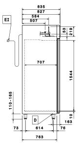
ED Remote electrical connection RO Refrigerant Outlet Electrical inlet (power) ΕI Refrigerant Inlet
